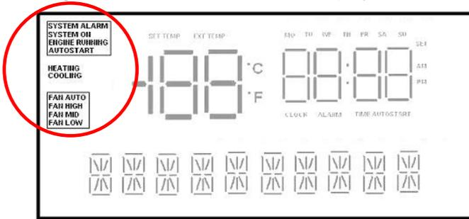
**SYSTEM ALARM** symbol will flash if an alarm condition has occurred. The alphanumeric display along the bottom of the display screen will show more information about the alarm. (Red status LED will be on.)
