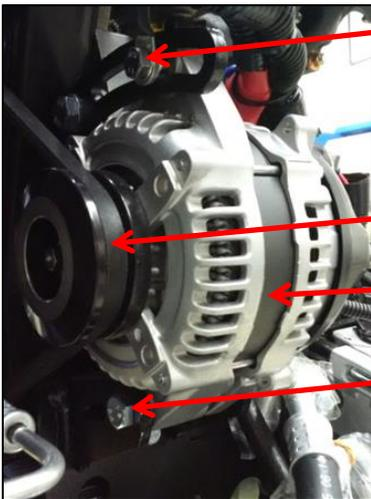
Alternator Adjuster Lock Bolt and Nut
