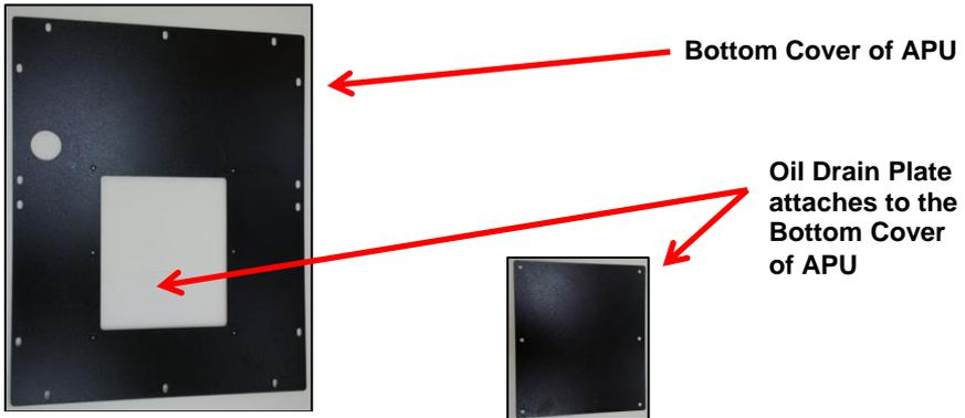
4. Remove the oil drain plate using a  $\frac{7}{16}$ " socket wrench from the bottom plate of the engine enclosure.
