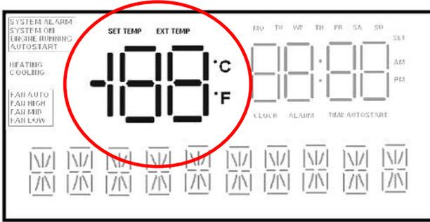
This area indicates the internal (or external) temperature and can be programmed to display in either “Celsius” or “Fahrenheit”.
