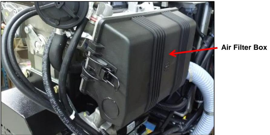
**Procedure to Replace the Air Filter**
